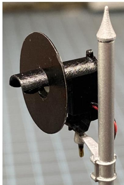
The last step is the target. This is cut to fit and slips over the lens assembly.
