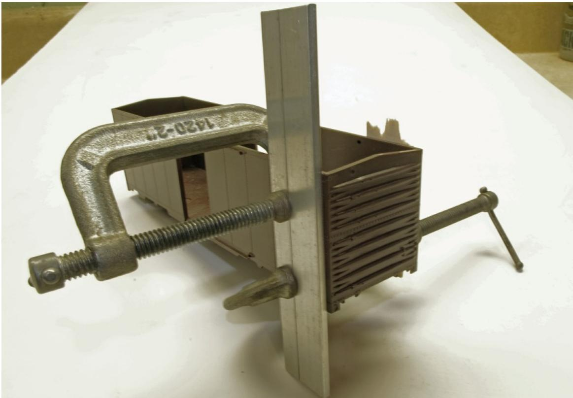
Use as straight guide to make sure your cut is straight and where it needs to be. The straight guide is lined up on the side of the car right where the side ends and the end of the car begins. Put a pad on the other side of the car so your clamp will not leave a mark on the side of the car.
