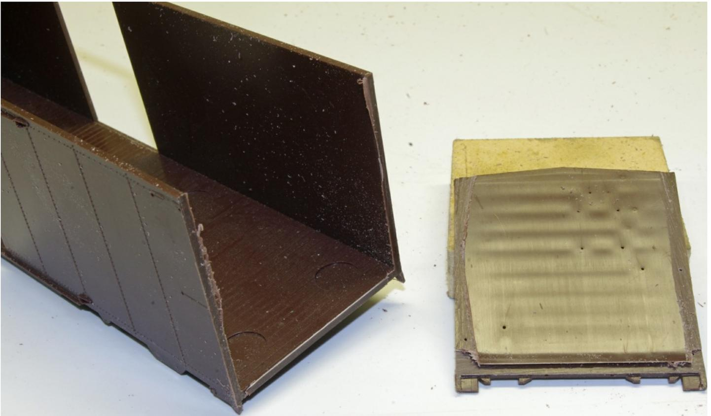
This is what your car should look like at this point. The cut is clean and straight. Clean up the flash with sand paper or a file. Check the fit of the end to see if there is any additional clean up. Clean up the end and touch up any flash that may be there.
