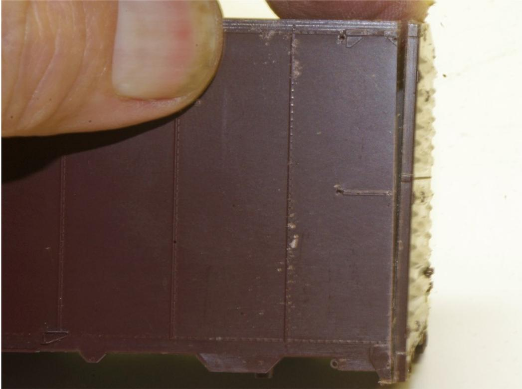
Take your time cutting and clean the plastic out of the saw teeth after a few strokes. When you have cut through like this stop and do the other side.
