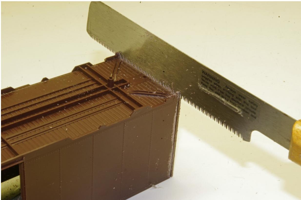
After you have cut through each side turn the car over and cut through the floor as shown. Use the side cuts as a guide. Keep the saw teeth clean or you will catch on the thin side of the car and break a corner off.
