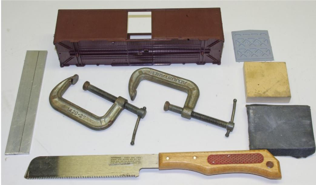
To install the Deco end on the car you will need to cut off the existing molded plastic end. The photo shows the tools you will need. The saw is a course tooth that cuts on the pull stroke. Any razor saw will work.
