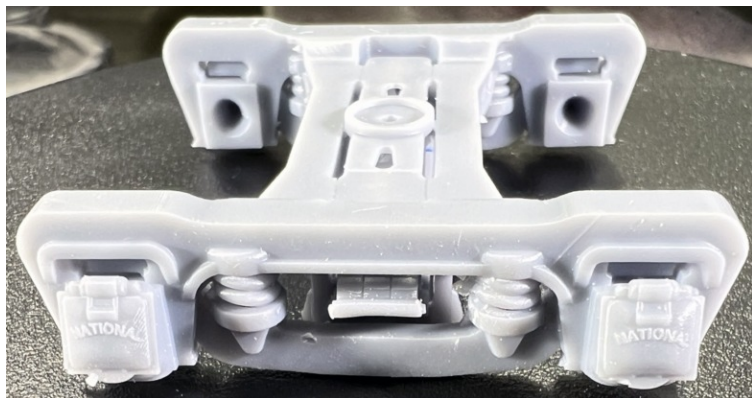
Above: Erie Express Trucks: The Erie Railroad used these General Steel Casting trucks under their milk cars and Caboose. Below: Diesel locomotive seats. Files from trainkitchen.com .
