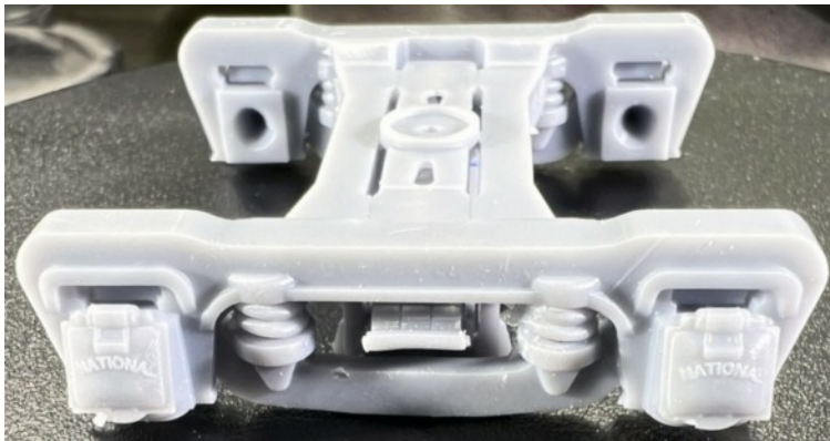
Above: Erie Express Trucks: The Erie Railroad used these General Steel Casting trucks under their milk cars and Caboose. Below: Diesel locomotive seats. Files from trainkitchen.com .
