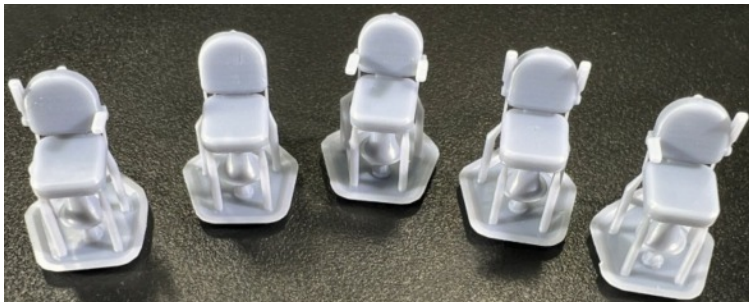
S scale Vulcan truck direct burnout from castable resin.
