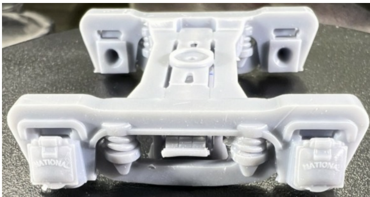
Above: Erie Express Trucks: The Erie Railroad used these General Steel Casting trucks under their milk cars and Caboosees. Below: Diesel locomotive seats. Files from trainkitchen.com .
